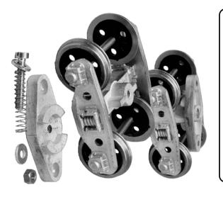
**BR Plate-Back Bogies Roller Bearing Axles**
