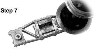
Offer up wheelset to check clearance. Make adjustments as required (possibly chamfer brake block rear with knife blade). When happy solder solid & clean up. Ensure rebate for stretcher end is clean & clear.
