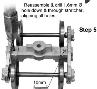
Cut from brass rod & fit assembly pins.
