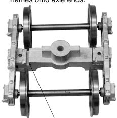
Note gap on stretcher when using Slater's wheelsets. My preferred solution is to reduce axle width by filing off the pin points (plus a couple of strokes) with a flat file.
