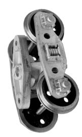
Bogies Fitted with Roller Bearing Designed for 3'1" wagon whee Later Design of BR Plate-Back
